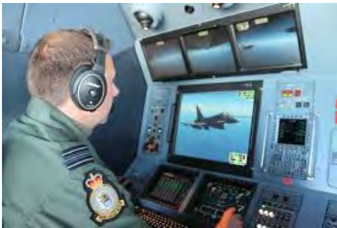
The Mission Systems Operator (MSO) controls the Air to Air Refuelling from his station behind the co-pilot
