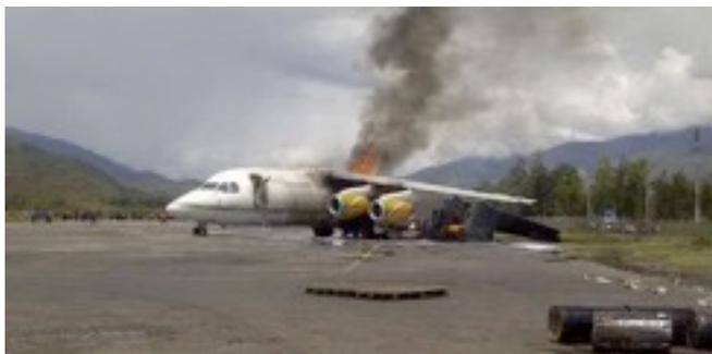
A Nusantara Air Charter British Aerospace BAe 146-200, registration PK-JKC performing a daily freight flight from Jayapura to Wamena (Indonesia) carrying fuel supplies for Wamena, had safely landed at Wamena, had reached its parking position, was shut down and being unloaded at around 11:50L (02:50Z), when one of the fuel drums caught fire and set the airplane ablaze. No injuries occurred, however, the aircraft burned down beyond repair.
