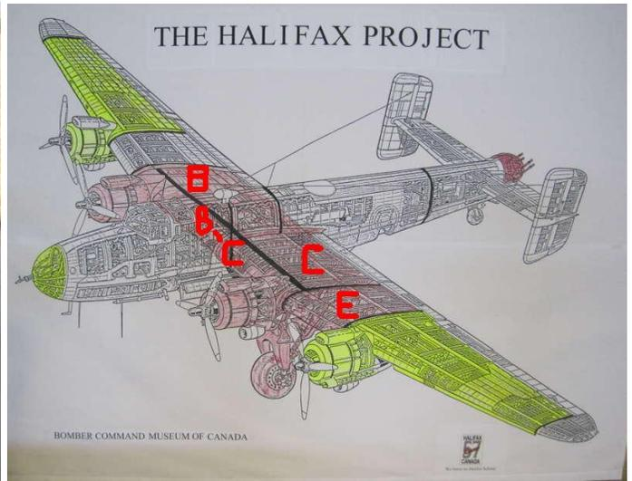
Remember that everything above (in light red) on the Halifax cutaway is what we have acquired and that which is (yellow) has been located. “B” is the right wing box and main spar, “C” is the left wing box and main spar, “E” is the intermediate wing section, and “B-C” is the middle main spar section. “A” and “D” are extra center section wings boxes we recovered. (We have the Boulton-Paul tail turret recovered from the UK and on display at the Bomber Command Museum of Canada in Nanton)
